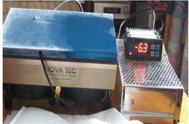
At the end of the lesson I sprayed the right side of the cold plate with a 23% sodium chloride brine and VOILA - the frost is eliminated immediately.
